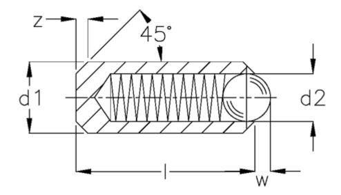
$\begin{array}{ll} \text{d1} & = 3.0 \\ \text{d2} & = 2.0 \\ \text{I} & = 7 \\ \text{Spring pressure N bottom} = 7.5 \\ \text{Spring pressure N top} & = 4.5 \\ \text{W} & = 0.65 \\ \text{z} & = 0.15 \end{array}$
